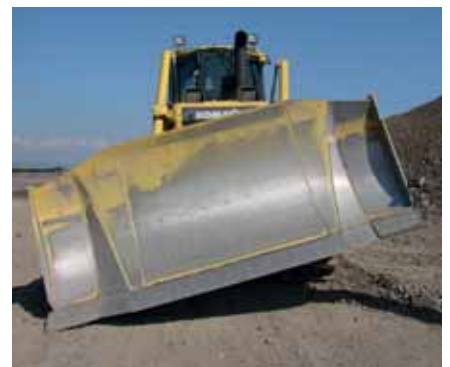
Hydraulically adjustable tilt: 870 mm
