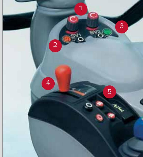
SV1/SV2 Speed memories (1), 'Pedal' or 'Lever' operating modes (2) and speed range selection (3) all in one convenient 'pod'
