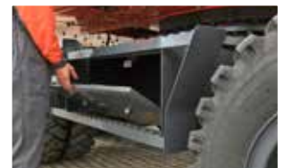
Tool box Lockable tool box on the right hand side.
