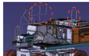
2 additional lateral safety bars With raised height for increased safety.
